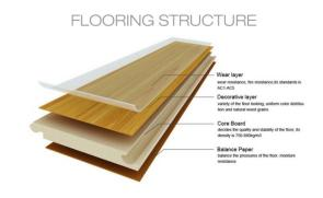
The photographic layer mimics the appearance of wood, stone, or tile, while the provides wear layer protection against stains and Particleboard scratches. or highdensity fiberboard often forms the core layer for added stability, with the backing layer enhancing support and moisture resistance.
